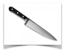
A wedge is made up of two inclined planes. The two planes meet and create a sharp edge. Wedges are used to push two objects apart, hold objects in place and cut an object into pieces. A knife is an example of a wedge with a sharp edge.
