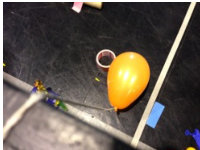
An extremely successful idea that we carried out, where a wind up car laden with unraveled safety pins hit the balloon, causing it to pop and let go of a marble using a balance beam at the top of a large box.
